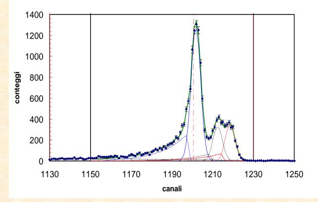
The off-line analysis of stored spectra, allows simple solution of interference problems.
