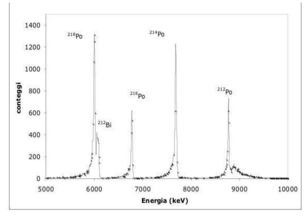
The interference between <sup>218</sup>Po line and <sup>212</sup>Bi line suggests to obtain radon concentration from the <sup>214</sup>Po line, but
