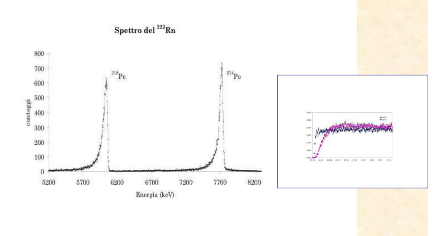
If this line could not be used, the use of <sup>214</sup>Po 7,7 MeV line makes this time of about 3 h, usually acceptable for geological applications
