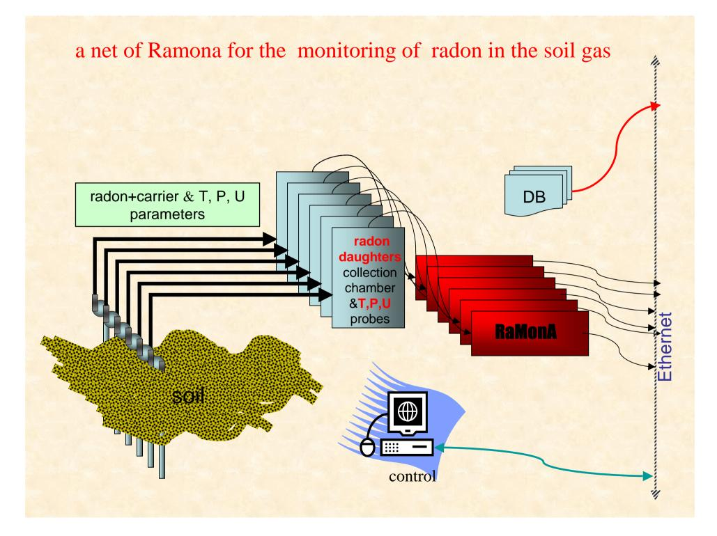
The **alpha particle spectrometry** on the gas coming directly from soil is the main peculiarity of this system. With this technique, in fact, which allows to detect independently radon and thoron daughters:
