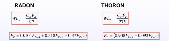
$F_R$  and  $F_T$  are equilibrium factors for Radon and Thoron progeny respectively, calculated with regard to the estimated extract ventilation rate.
