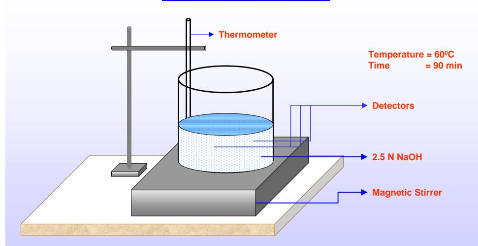
Latent tracks are enlarged to microscopically visible size by chemical etching.
