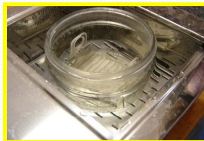
etching: NaOH 6M 98°C 1h
