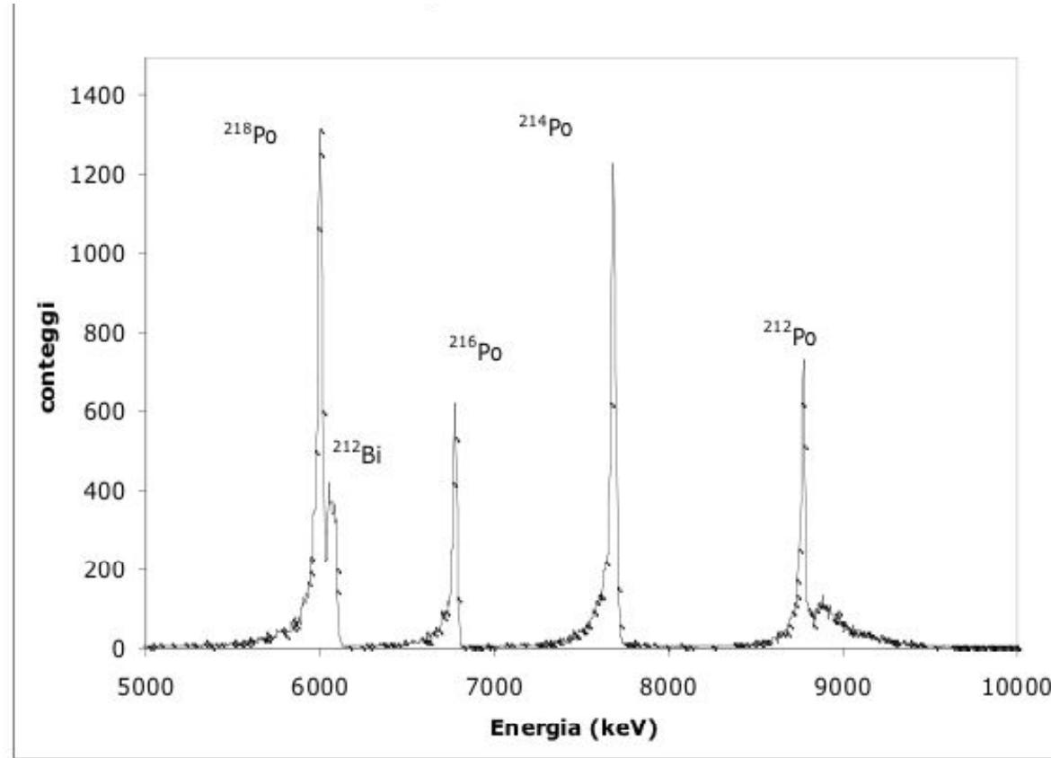
The interference between  $^{218}\text{Po}$  line and  $^{212}\text{Bi}$  line suggests to obtain radon concentration from the  $^{214}\text{Po}$  line, but ...
