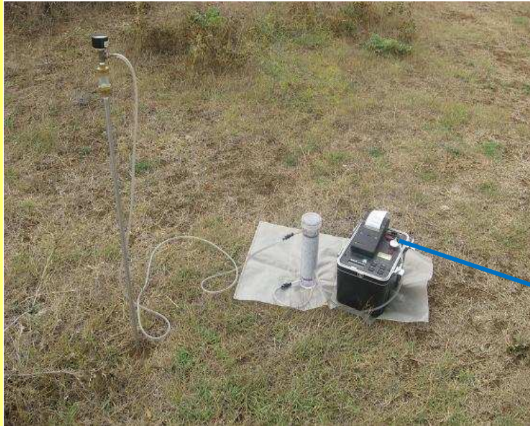
Air flow meter used to measure properly the RAD7 pump flux
