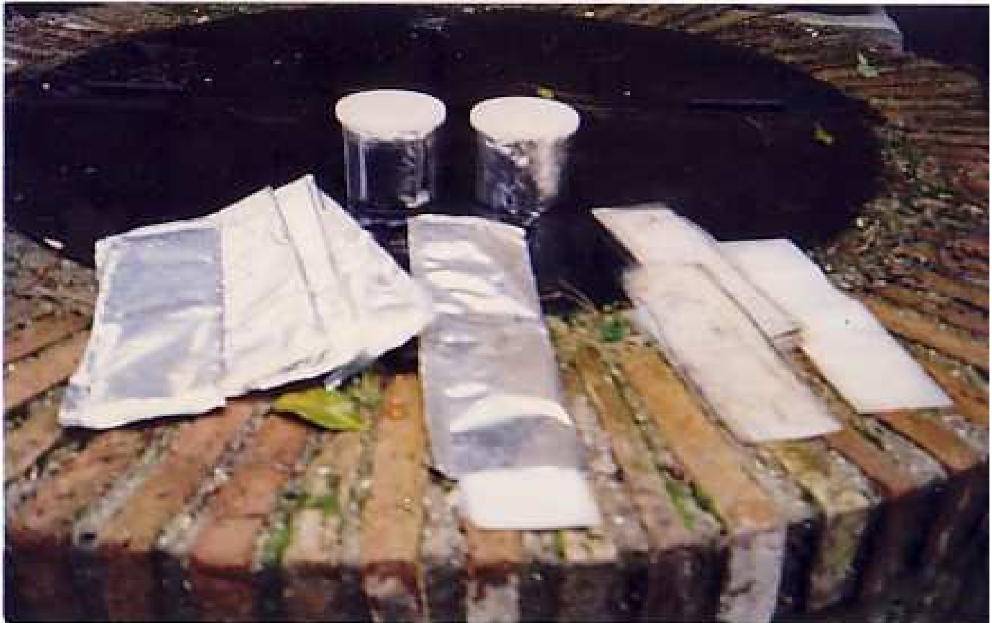
PE-films for in-water-radon sampling , followed by gamma spectrometry (Tommasino, 1998)
