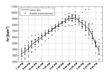
The **natural ventilation rate**  $\lambda$  can be measured fitting the accumulation/depletion branches of the curve, assuming K constant.
