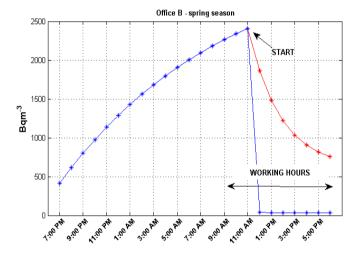
The mean concentration during working hours is not low because the first and second radon value (9:00 - 10:00 AM) before starting fan are very high.
