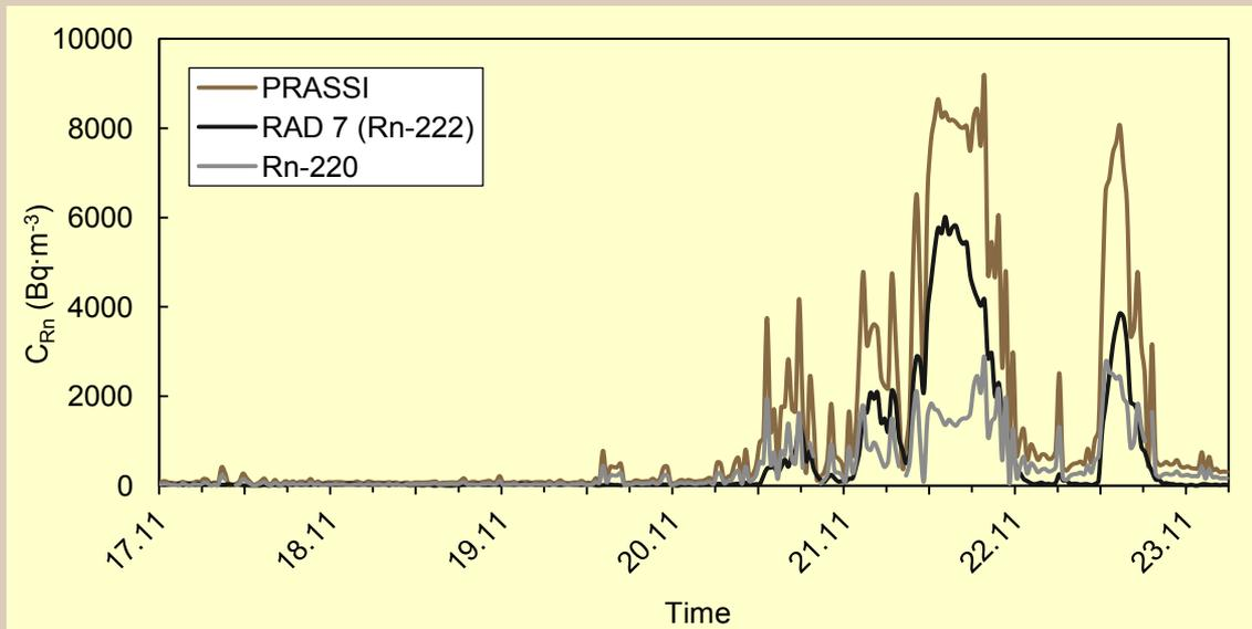
$$C_{Rn-20} = \frac{C_{Rn}^{PRASSI} - C_{Rn}^{RAD7}}{1.73}$$
