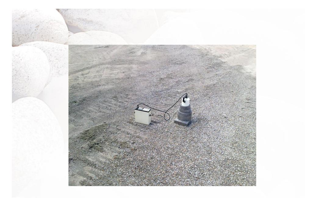
Regular background measurements on lead plate
