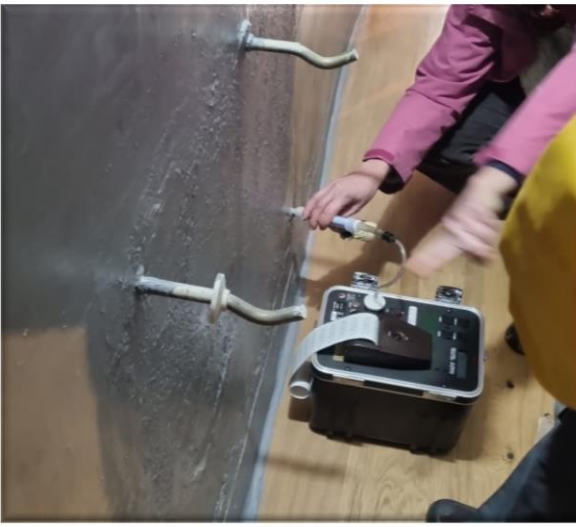
Measurements of radon entry points with RAD7 (Durrige Company Inc)
